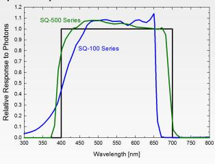
Mean spectral response measurements of six replicate Apogee SQ-100 and SQ-500 series quantum sensors. Spectral response measurements were made at 10 nm increments across a wavelength range of 300 to 800 nm in a monochromator with an attached electric light source. Measured spectral data from each quantum sensor were normalized by the measured spectral response of the monochromator/electric light combination, which was measured with a spectroradiometer.
