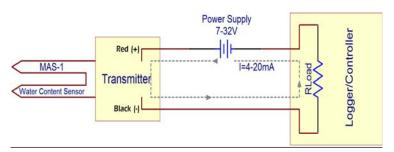
Figure 1 - 4-20mA current loop diagram
