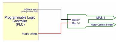
Figure 2 - Typical wiring connection
