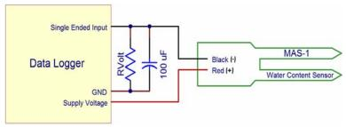
Figure 3 - Wiring connection for devices without current inputs
