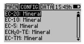
To modify a sensor's calibration type, press **ENTER.** You can choose a preset soil calibration type or create your own (See creating a Custom Calibration). To change the soil calibration type, press **ENTER** when the medium option is selected. You can view the calibration coefficients by pressing **ENTER** when the coefficients option is highlighted. Press **SAVE** to save your calibration preference or press **ESC** to exit without saving changes.
