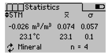
Use the arrows to select the correct sensor. When you press Enter, the connected sensor will show you the current reading on the left hand side of the screen.
