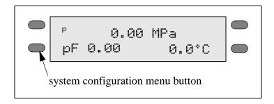
You can change how the beeper signals after each reading and enter the calibration menu as well.
