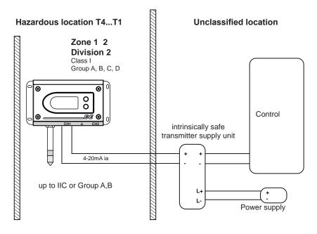
Example of EE300Ex mounting of remote sensing probe in Zone 0 or Division 1 and transmitter in Zone 1 or 2 or Division 2
