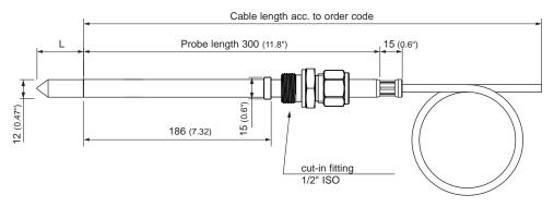
Remote sensing probe humidity/temperature up to 20bar (300psi) or 300 bar (4351 psi) - Model E and M
