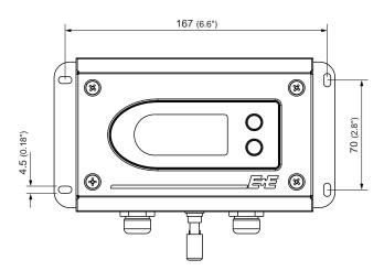
The lower housing section is mounted using 4 screws. Screw diameter < 4.5mm (0.18")
