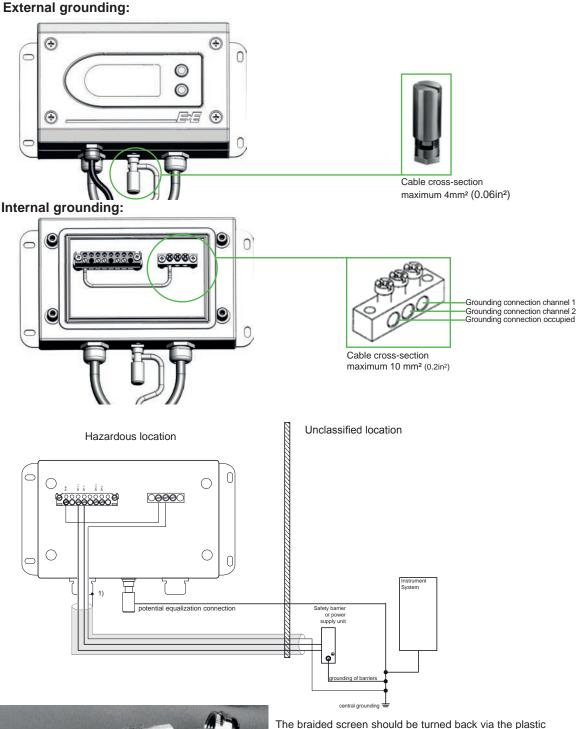
insert on the cable connection. The introduction of the plastic insert presses the braided screen onto the interior
