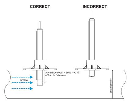
When installing the EE671 probe without the mounting flange, make sure that the arrow on the sensing head matches exactly the flow direction.
