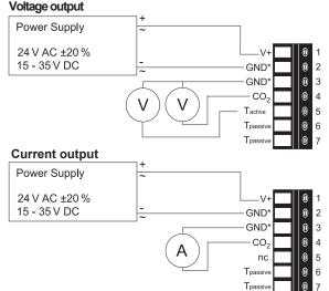
\* Very important: for failure-free operation and performance according to the specs the supply GND and the measurement GND must be wired separately.
