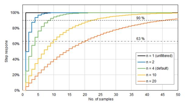
Fig. 13 Step response vs. samples
