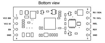
Fig. 6 Pin assignment
