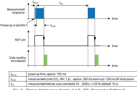
Fig. 7 Timing details (see chapter 4.4.3: "CO<sub>2</sub> Parameter Settings")
