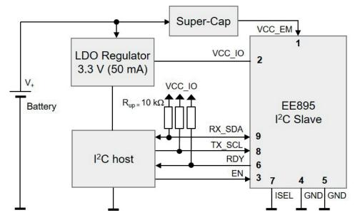
Fig. 11 Example battery powerd devices
