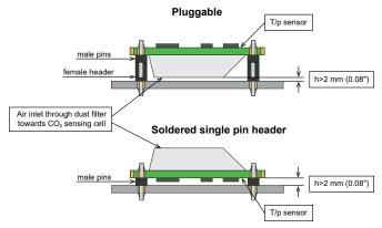
Fig. 3 Mounting with soldered pin header
