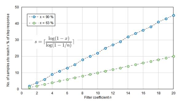
Fig. 14 Step response vs. filter coefficient
