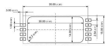
Fig. 2 Recommended PCB footprint
