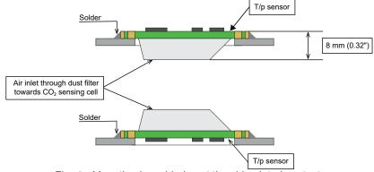
Fig. 4 Mounting by soldering at the side plated contacts
