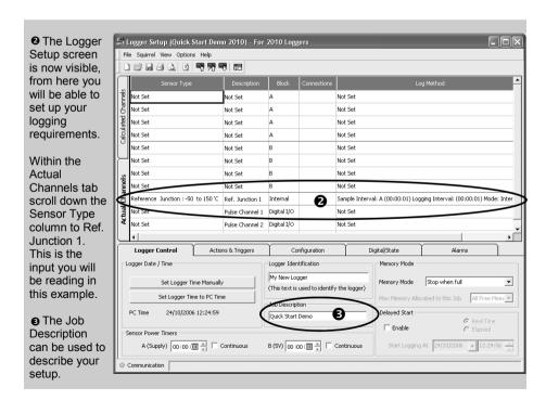
O Click to send setup to logger and start logging. Let the unit log for a few minutes.
