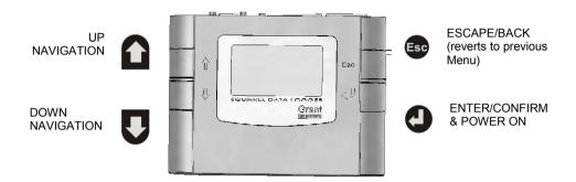
To use the 2010 control panel press , the opening display will be shown (see right). The display timeout is preset to 10 seconds, however this can be changed by selecting the Configuration tab within the Logger Setup window of SquirrelView.
