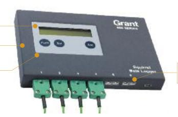
Automatically detects when sensors are present - easy set-up of up to 6 channels
