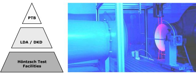
Free jet wind tunnel WK320 with laser Doppler anemometer (LDA)
