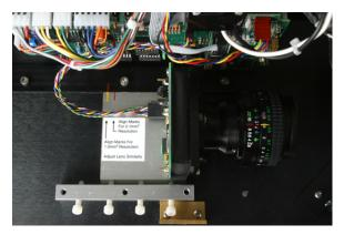
**Figure 7.** LI-3100C camera position configured for 1.0 mm<sup>2</sup> operation.
