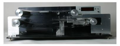
**Figure 9.** Upper belt rocking idler and lower belt idler removed. To remove the belts, draw them outward.
