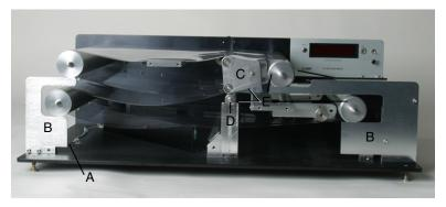
**Figure 8.** LI-3100C with front plate removed. (A) Fluorescent tube power connector, (B) pulley support brackets, (C) upper belt rocking idler, (D) lower belt idler, (E) proper location of pulley peripheral end grooves, lower belt idler peripheral end groove, and the end plate notch.
