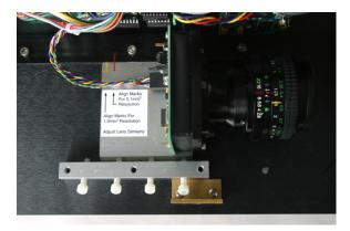
**Figure 6.** LI-3100C camera position configured for 0.1 mm<sup>2</sup> operation.
