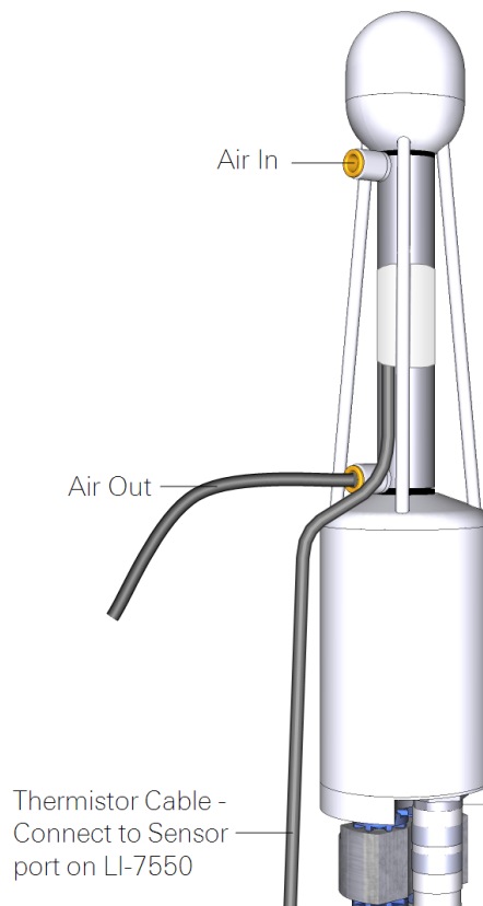
Figure 4-1. Flow calibration gas into the calibration fitting. Attach a 15 cm (6 in.) piece of tubing to the outlet to prevent diffusion of ambient air into the calibration fitting.
