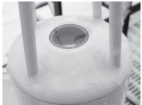
Figure 5-1. Water on the sapphire windows can cause low signal strength (formerly AGC) values.
