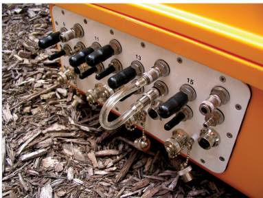
Figure 6. In the absence of extension tubing, the leak test fixture is attached between the air inlet and outlet ports (port #14 shown).
