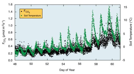
An example of time series data for soil  $CO_2$  flux  $(F_{CO_2})$  obtained with a 16-chamber system at Lincoln, Nebraska. Soil temperature data at a depth of 5 cm from each chamber are also shown. For more information on data collected from a multiplexed system, visit www.licor.com/multiplex.
