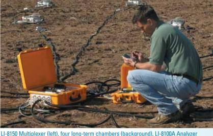
LI-8150 Multiplexer (left), four long-term chambers (background), LI-8100A Analyze Control Unit (right), communication through wireless PDA.
