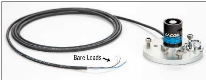
Figure 2-4. LI-190R-BL Quantum Sensor featuring 3-wire bare leads.
