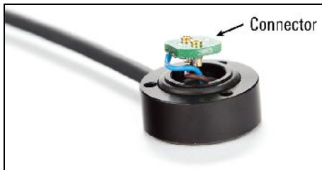
Figure 6-2. Sensor base and cable assembly with sensor head removed.
