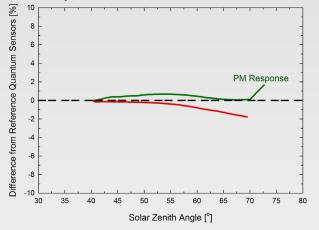
Mean cosine response of seven Apogee MQ-510 quantum sensors. Cosine response measurements were made on the rooftop of the Apogee building in Logan, UT. Cosine response was calculated as the relative difference of MQ-510 quantum sensors from the mean of replicate reference quantum sensors (LI-COR models LI-190 and LI-190R, Kipp & Zonen model PQS 1). The red data are AM measurements; the green data are PM measurements.
