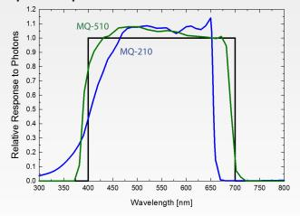
**Spectral Errors of Commercial Quantum Sensors**
