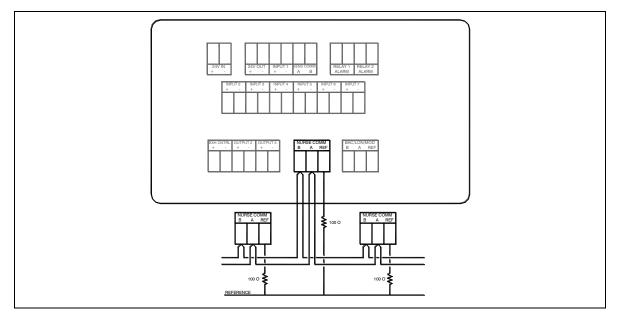
Figure 37. Wiring Diagram – Optional Nurses Station Communications Wiring to Model RPC30
