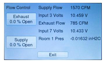
Figure 13. Flow Control screen in Diagnostics menu
