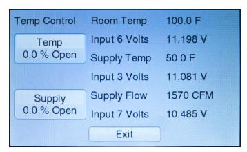
Figure 14. Temp Control screen in Diagnostics menu
