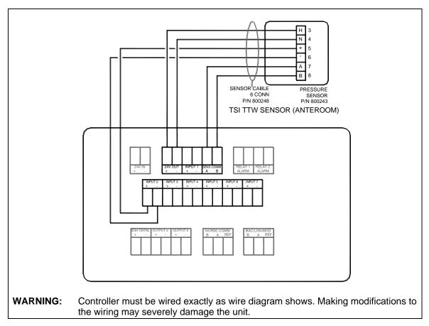
Figure 20: Optional Anteroom Through-The-Wall Sensor Wiring to Model RPC30
