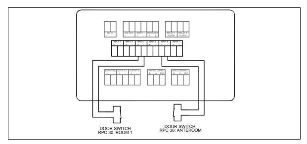
Figure 27. Optional Door Switch Wiring to Model RPC30
