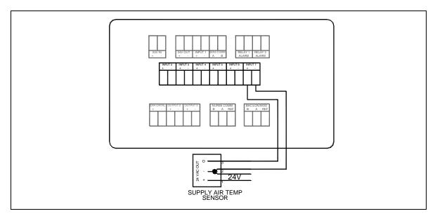
Figure 34. Optional Supply Air Temperature Sensor Wiring to Model RPC30
