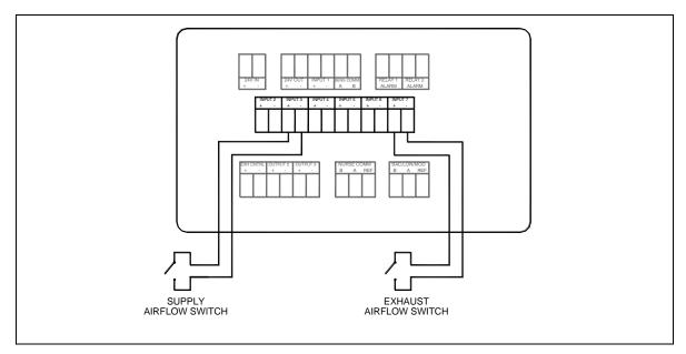
Figure 23. Optional Supply & Exhaust Flow Switch Wiring to Model RPC30
