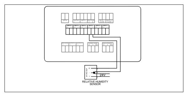
Figure 32. Optional Relative Humidity Sensor Wiring to Model RPC30
