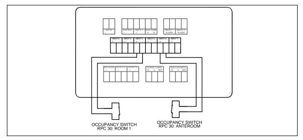
Figure 28. Optional Occupancy Sensor Wiring to Model RPC30
