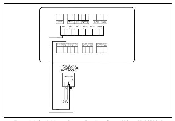
Figure 22. Optional Anteroom Pressure Transducer Sensor Wiring to Model RPC30
