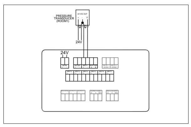
Figure 21. Wiring Diagram – Pressure Transducer Sensor to Model RPC30
