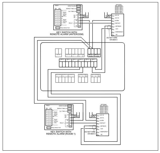
Figure 31. Optional Keyswitch with Remote Alarm Wiring to Model RPC30
