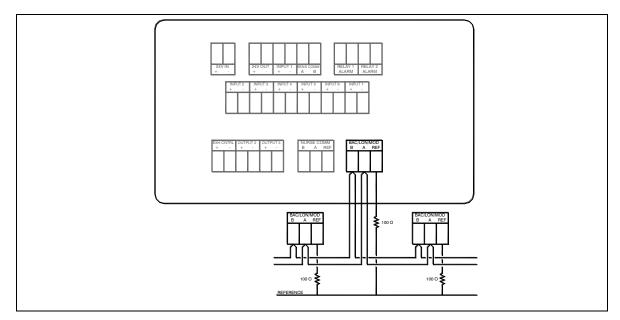
Figure 38. Optional Modbus and BACnet MS/TP Communications Wiring to Model RPC30
