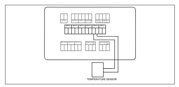
Figure 29. Optional Temperature Sensor Wiring to Model RPC30
