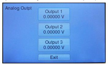
Touch the Output 1, Output 2, Output 3 button to manually set the output signal.
