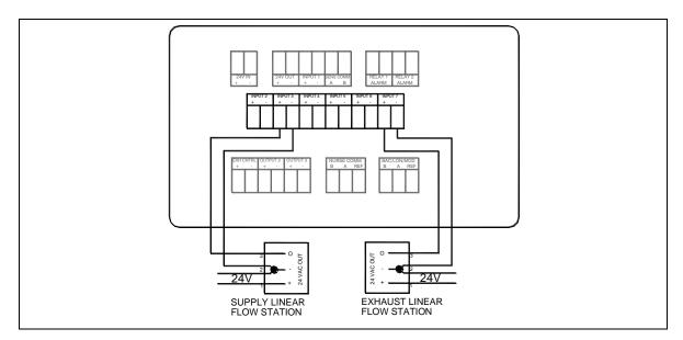
Figure 25. Optional Supply & Exhaust Linear Flow Station Wiring to Model RPC30
