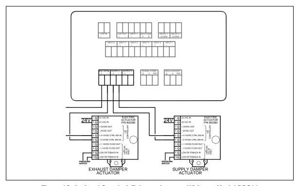
Figure 35. Optional Supply & Exhaust Actuator Wiring to Model RPC30
