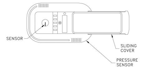
Figure 12: Pressure sensor door slid open
