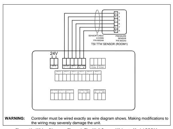
Figure 19: Wiring Diagram -Through-The-Wall Sensor Wiring to Model RPC30
